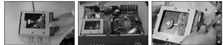
4. Install the HDD. Please note the HDD is placed upside down. Please make sure bracket is in correct position. 5. Fix the HDD bracket. 6. Connect to SATA port
