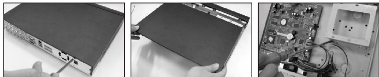
1. Loosen the screw s 2. Remove the upper cover of the DVR 3. Dismantle the HDD bracket
