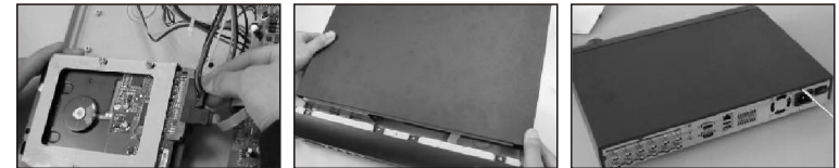
7. Connect to HDD power cable. 8. Place upper cover back. 9. Screw the upper cover firmly.
