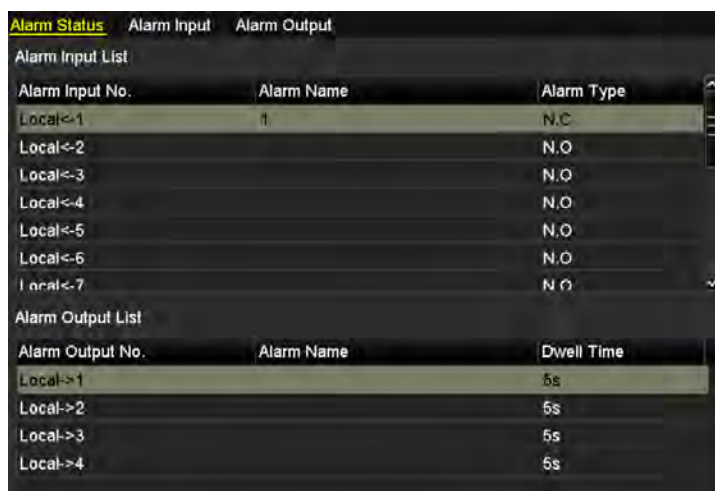
Figure 8. 5 Alarm Status Interface of System Configuration
