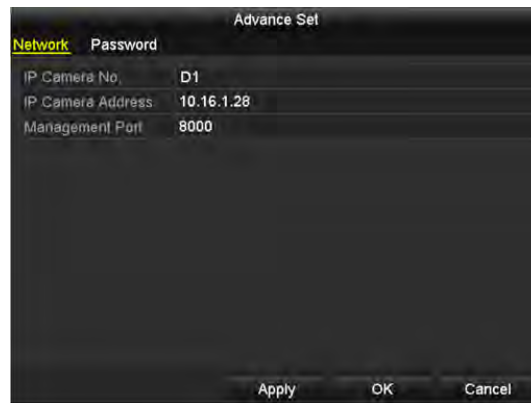
Figure 2. 18 Network Configuration of the Camera
