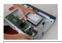
4. Place the HDD in accordance with the four holes.
