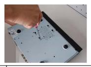
6. Fix the HDD firmly.
